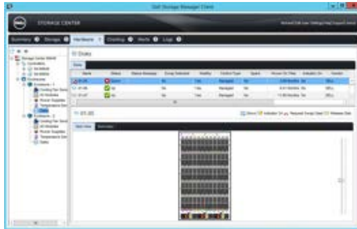
Figure 33. Disk View Showing the Failed Hard Drive
