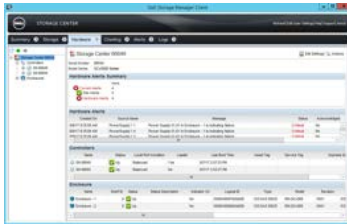
Figure 45. Hardware Alert Identifying the Expansion Enclosure with the Failed Power Supply
