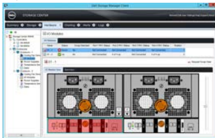
Figure 42. Rear View of the Expansion Enclosure Showing the Failed EMM
