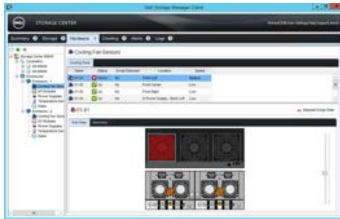
Figure 38. Rear View of the Expansion Enclosure Showing the Failed Cooling Fan Module
