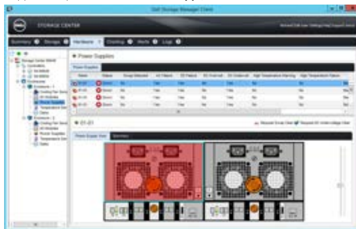
Figure 46. Rear View of the Expansion Enclosure Showing the Failed the Power Supply
