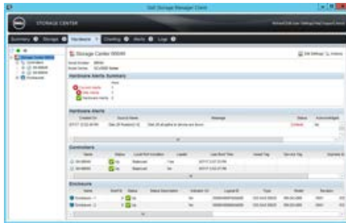
Figure 32. Hardware Alert Identifying the Expansion Enclosure with the Failed Hard Drive
