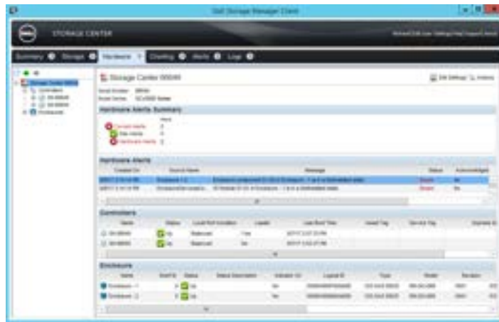
Figure 41. Hardware Alert Identifying the Expansion Enclosure with the Failed EMM
